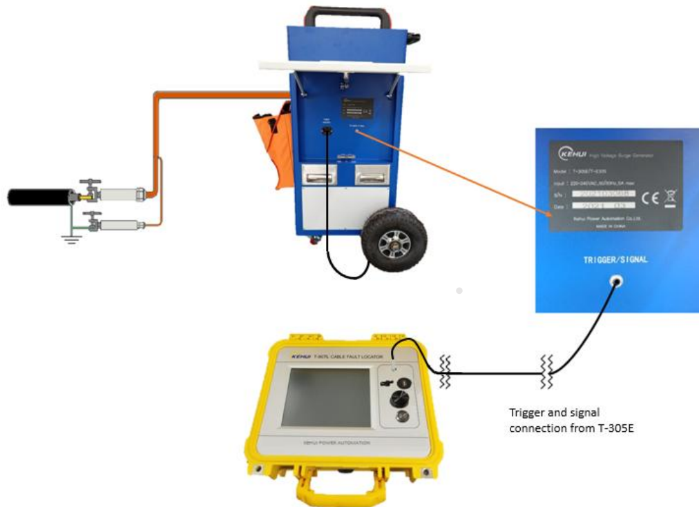
Figure 5.4 ICM set-up using T-305E
