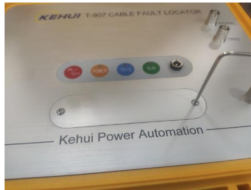
Figure A1.1 Opening the battery box
