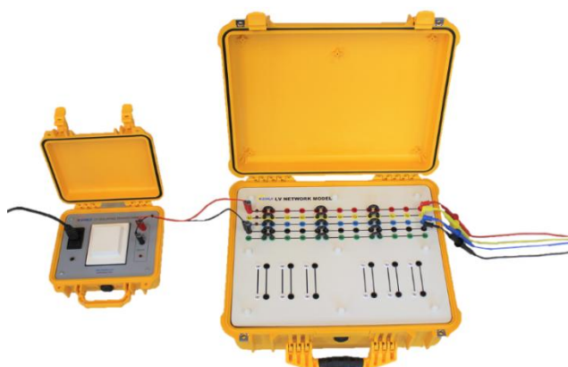
Network simulator energised by the T-MNS1 isolating transformer.
