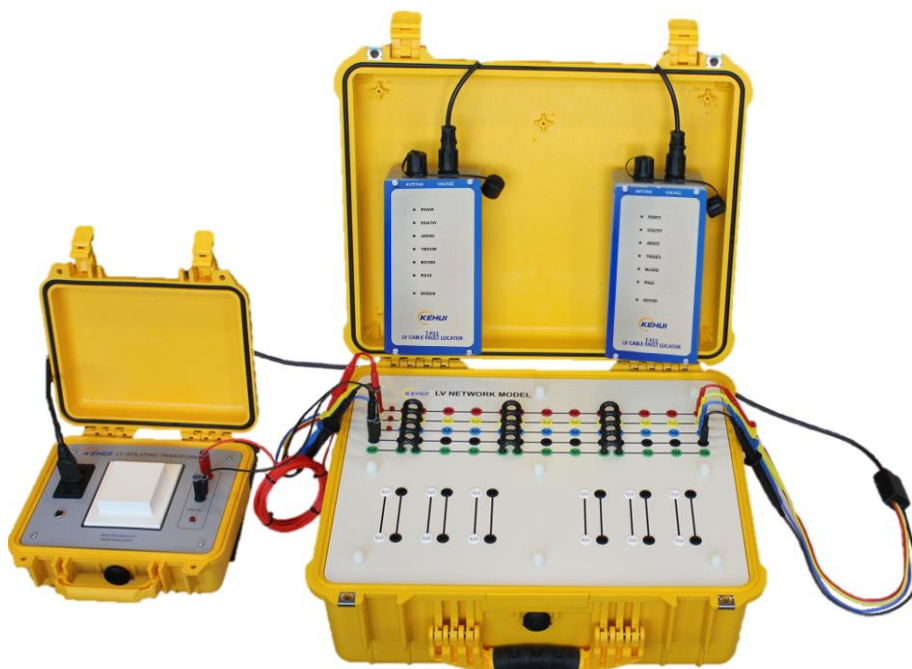
Figure 8.1: Connection of T-NM1 Network Model connected to test TRS scheme
