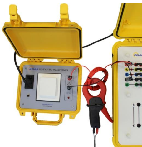
Figure 6.3 – T-NM1 with current connection for T-P22
