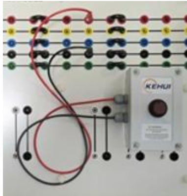
Figure 8.5 Applying a fault to the TRS scheme using the push-button
