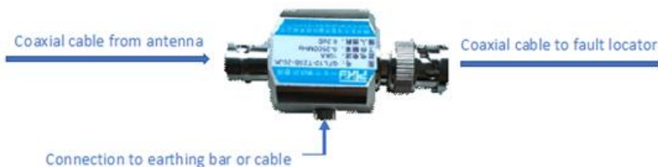
Figure 4.12 Surge protective device (SPD)
