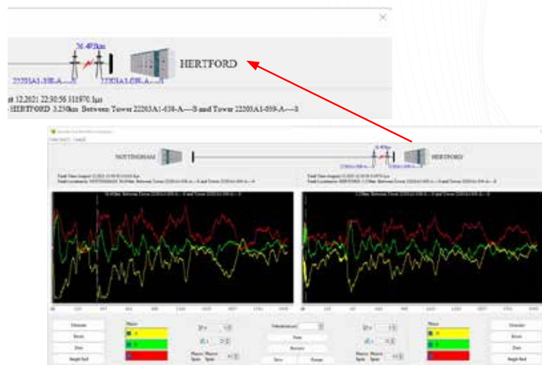
Waveform trace with automatic fault location
